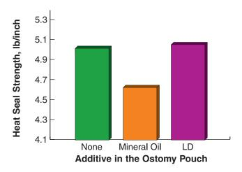
Lubricating Deodorant (LD) does not attack and weaken the heat seals of the pouch, unlike mineral oil. The heat seal strength of the pouch treated with Lubricating Deodorant (LD) is comparable to the untreated control (no additive).
